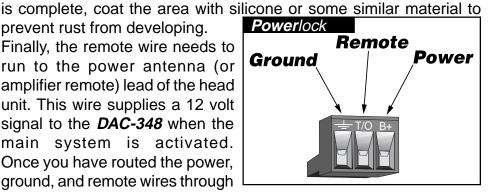
the vehicle, it is time to connect the wires to the DAC-348. Be sure that you have not reconnected the ground cable to the negative post of the battery.
